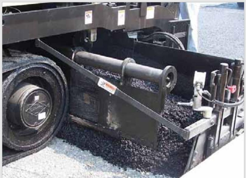
*End gate no more than 450 mm from the end of the auger and auger tunnel.*
