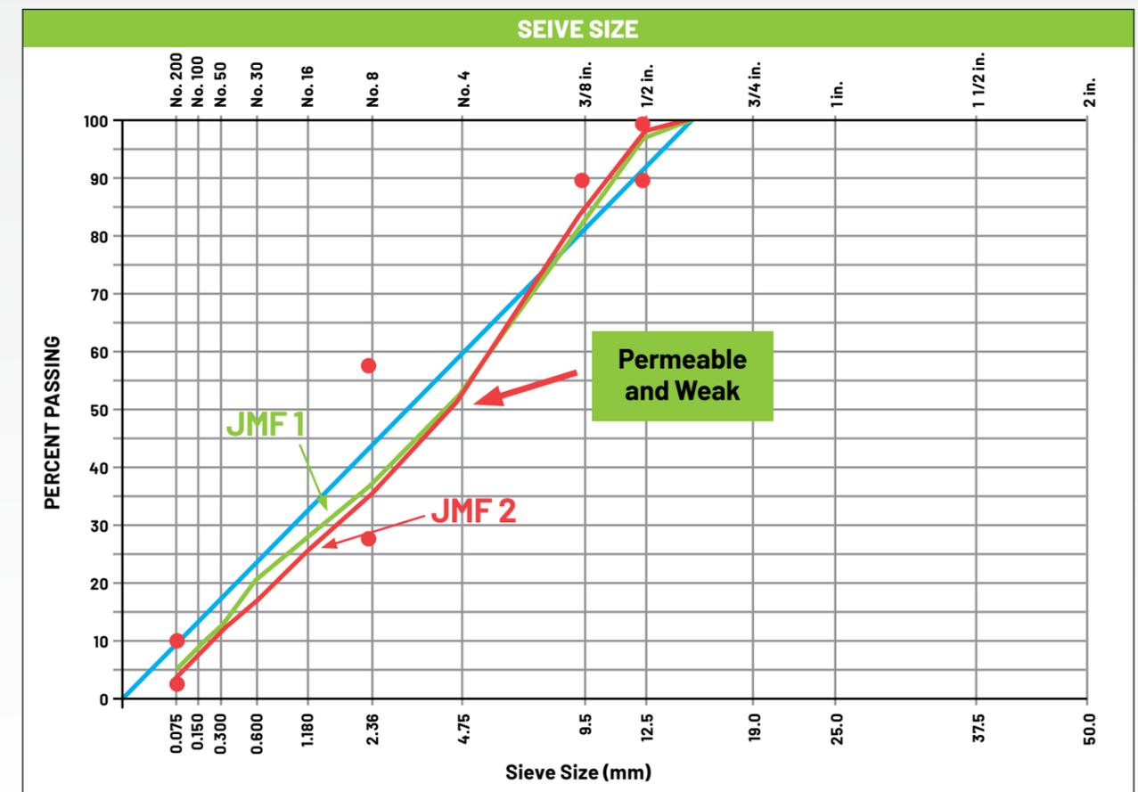
Figure 2 Example of Coarse Gradation
