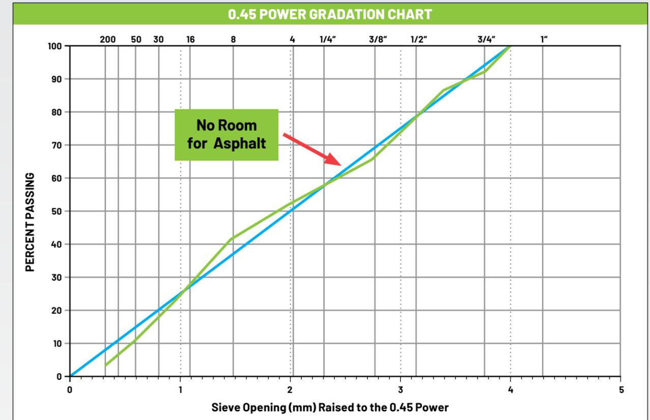
Figure 1 Example of Dense-Packed Gradation
