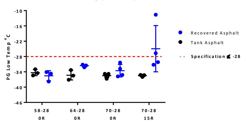
0% of tank samples failed 14 % recovered asphalt failed
