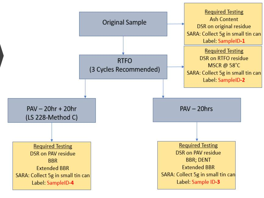
Testing Flow Chart: Sample D Recovered Asphalt
