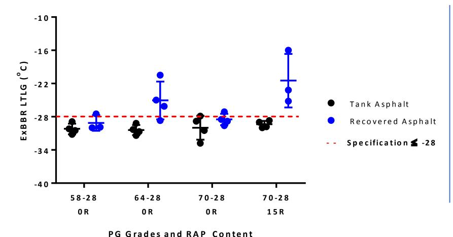
6% of tank samples failed 57% recovered samples failed
