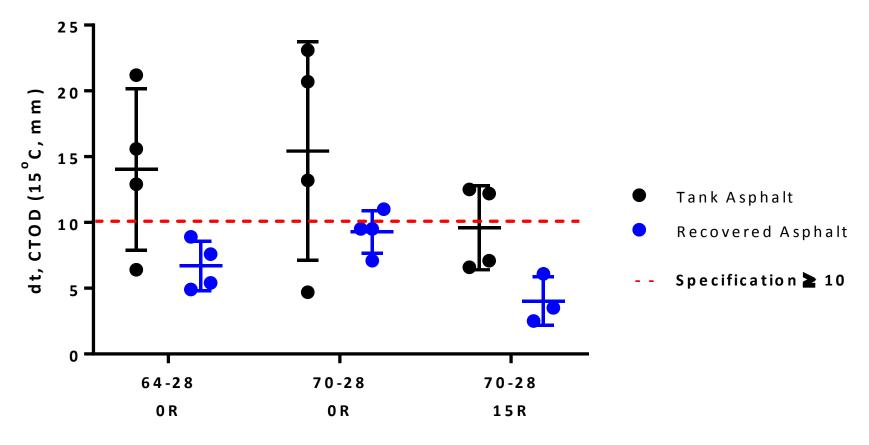
33% of tank samples failed 90% recovered samples failed
