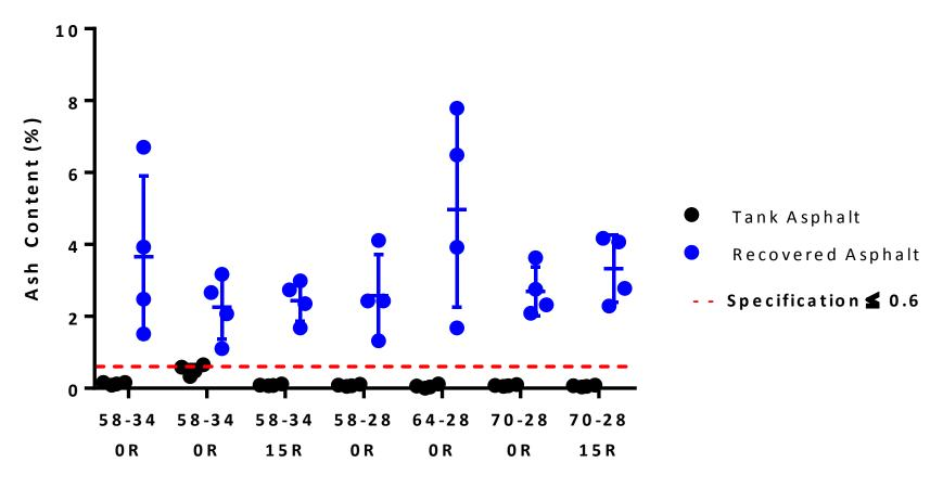
0% of tank samples failed 100% recovered asphalt failed
