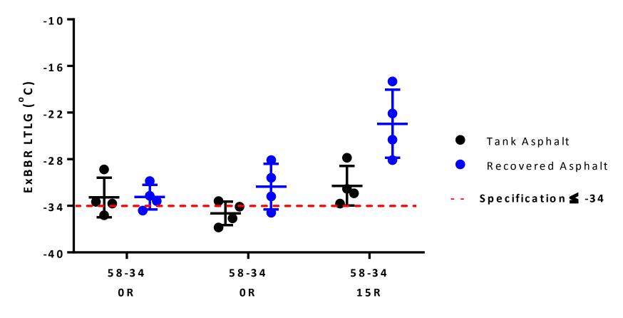
67% of tank samples failed 83% recovered samples failed
