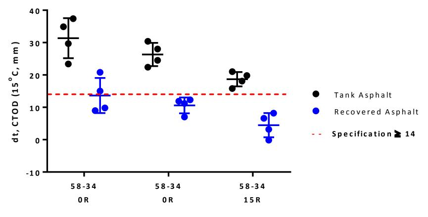
0% of tank samples failed83% recovered samples failed
