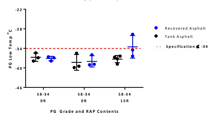
0% of tank samples failed 11% recovered asphalt failed
